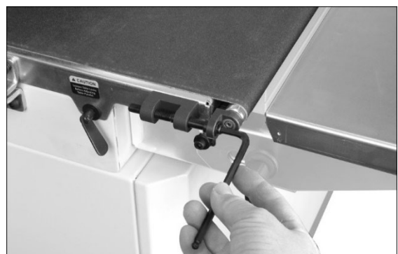
Figure 8-3: belt tension adjustment
